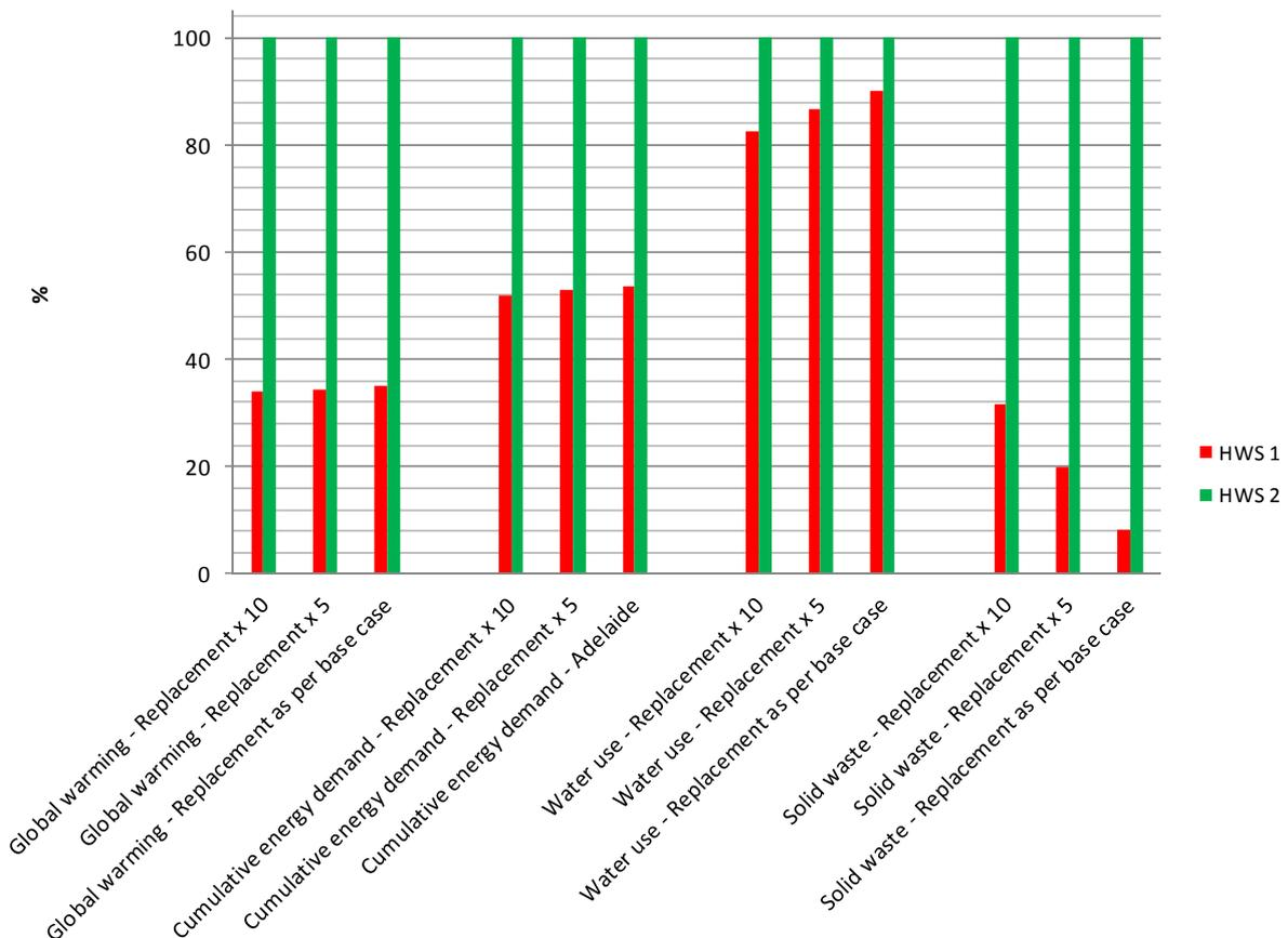
Figure 6-19: Relative summary of sensitivity of replacement, materials & building life results for La Banque (scaled from highest impact) red bar HWS1, green bar HWS2
