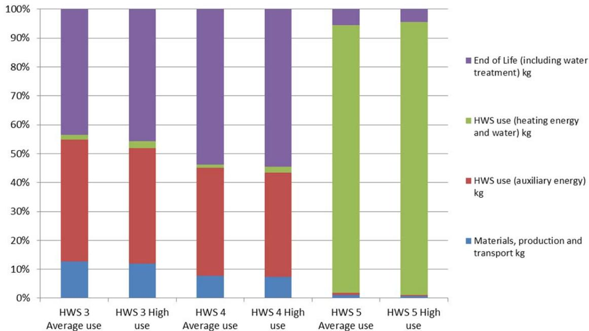
Figure 6-8: Disaggregated % characterisation results for solid waste for Brahe Place HWSs
