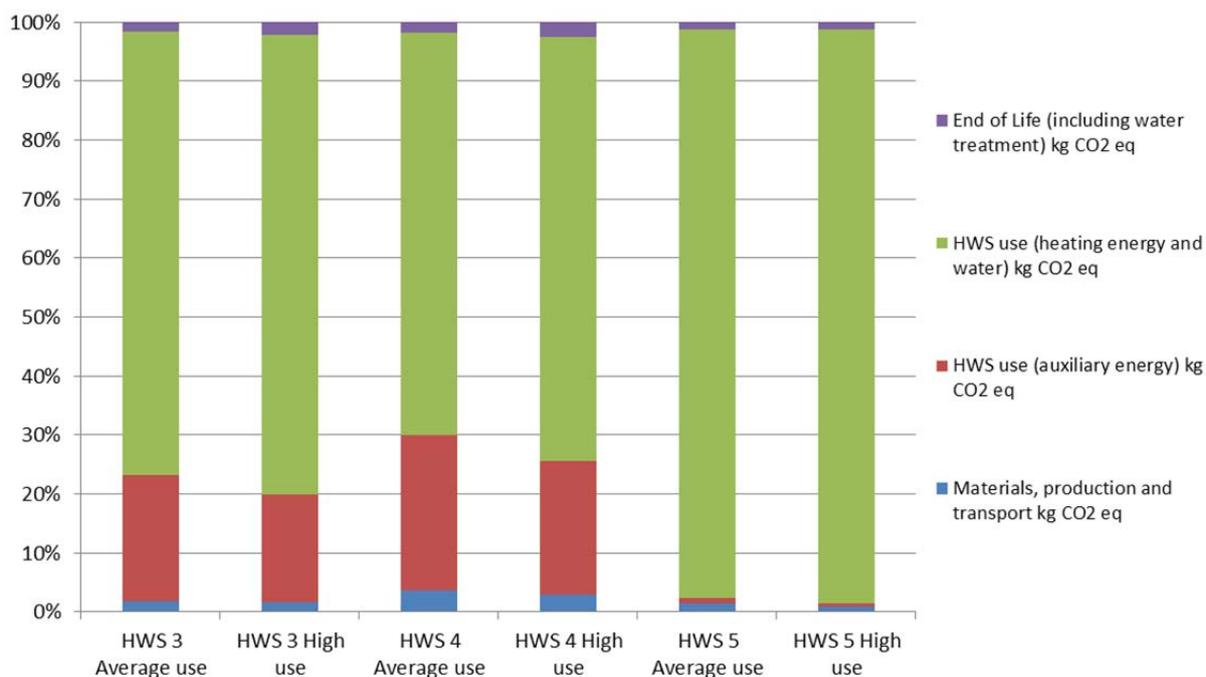
Figure 6-5: Disaggregated % characterisation results for global warming potential for Brahe Place HWSs
