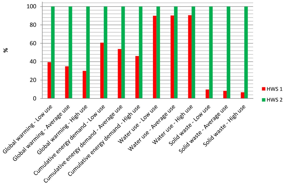
Figure 1: Relative summary of characterised results for La Banque (scaled from highest impact) red bar HWS1, green bar HWS2
