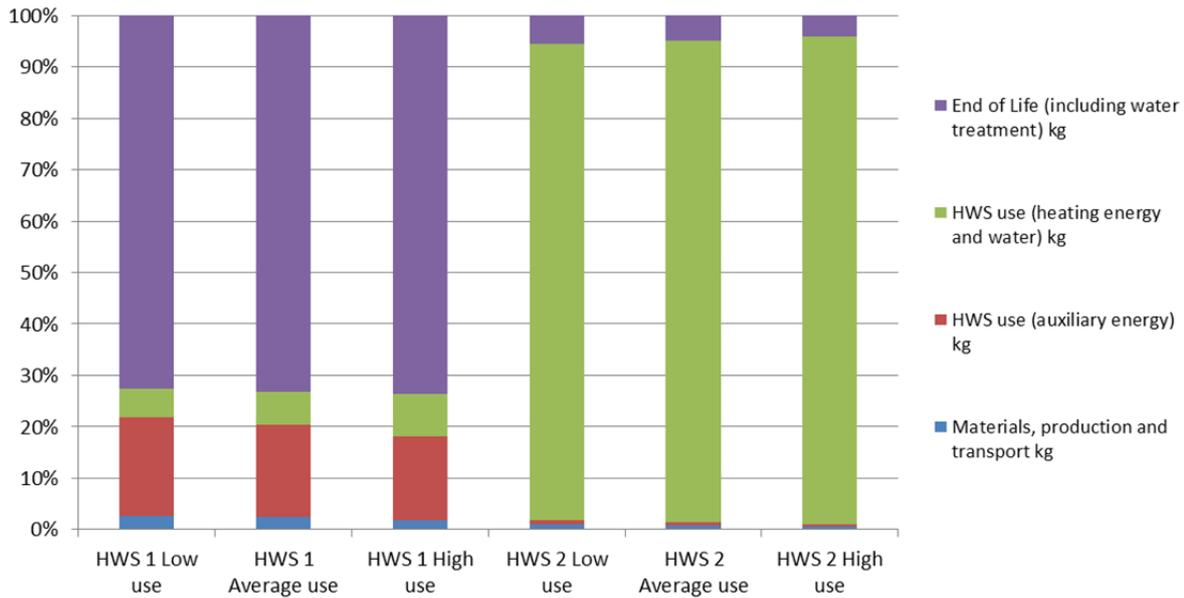
Figure 6-4: Disaggregated % characterisation results for solid waste for La Banque HWSs
