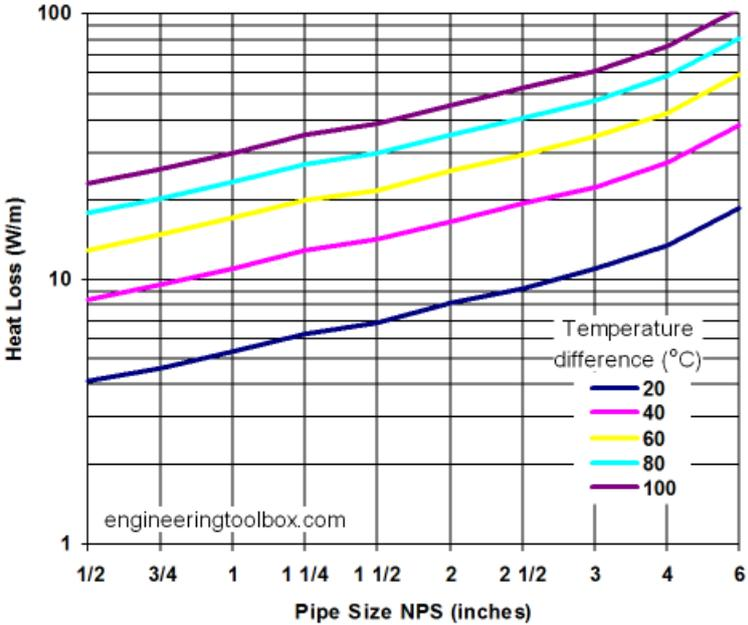
Figure 4-9: Heat loss in pipes for insulation 25 mm thick (The Engineering ToolBox 2012)
