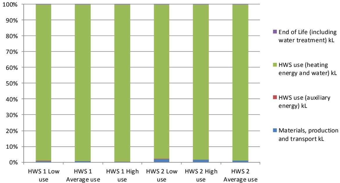
Figure 6-3: Disaggregated % characterisation results for water use for La Banque HWSs
