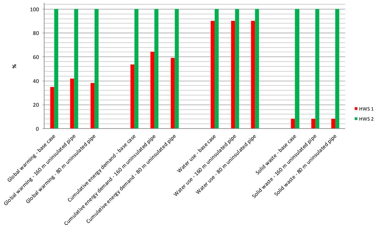
Figure 6-22: Relative summary of sensitivity of extra centralised system loss results for La Banque (scaled from highest impact) red bar HWS1, green bar HWS2
