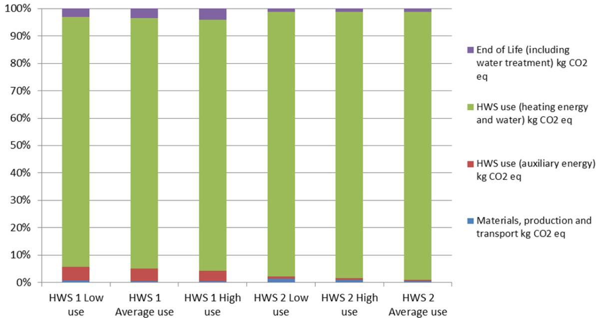
Figure 6-1: Disaggregated % characterisation results for global warming potential for La Banque HWSs
