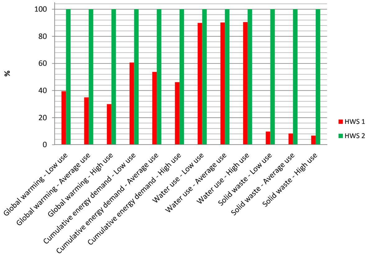
Figure 5-1: Relative summary of characterised results for La Banque (scaled from highest impact) red bar HWS1, green bar HWS2
