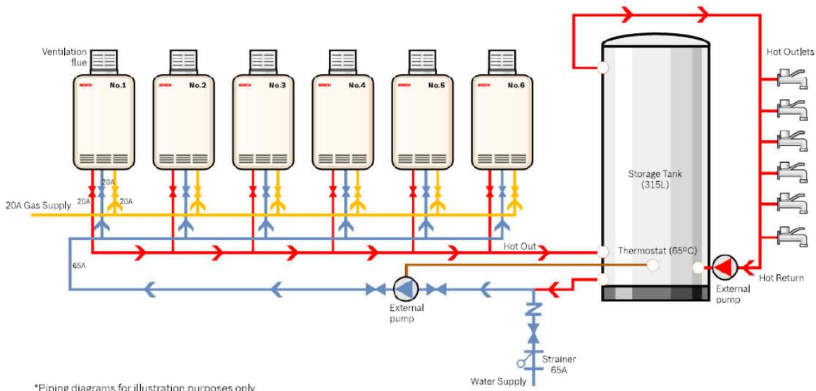
Figure 4-10: Typical ring main setup (Bosch 2011)
