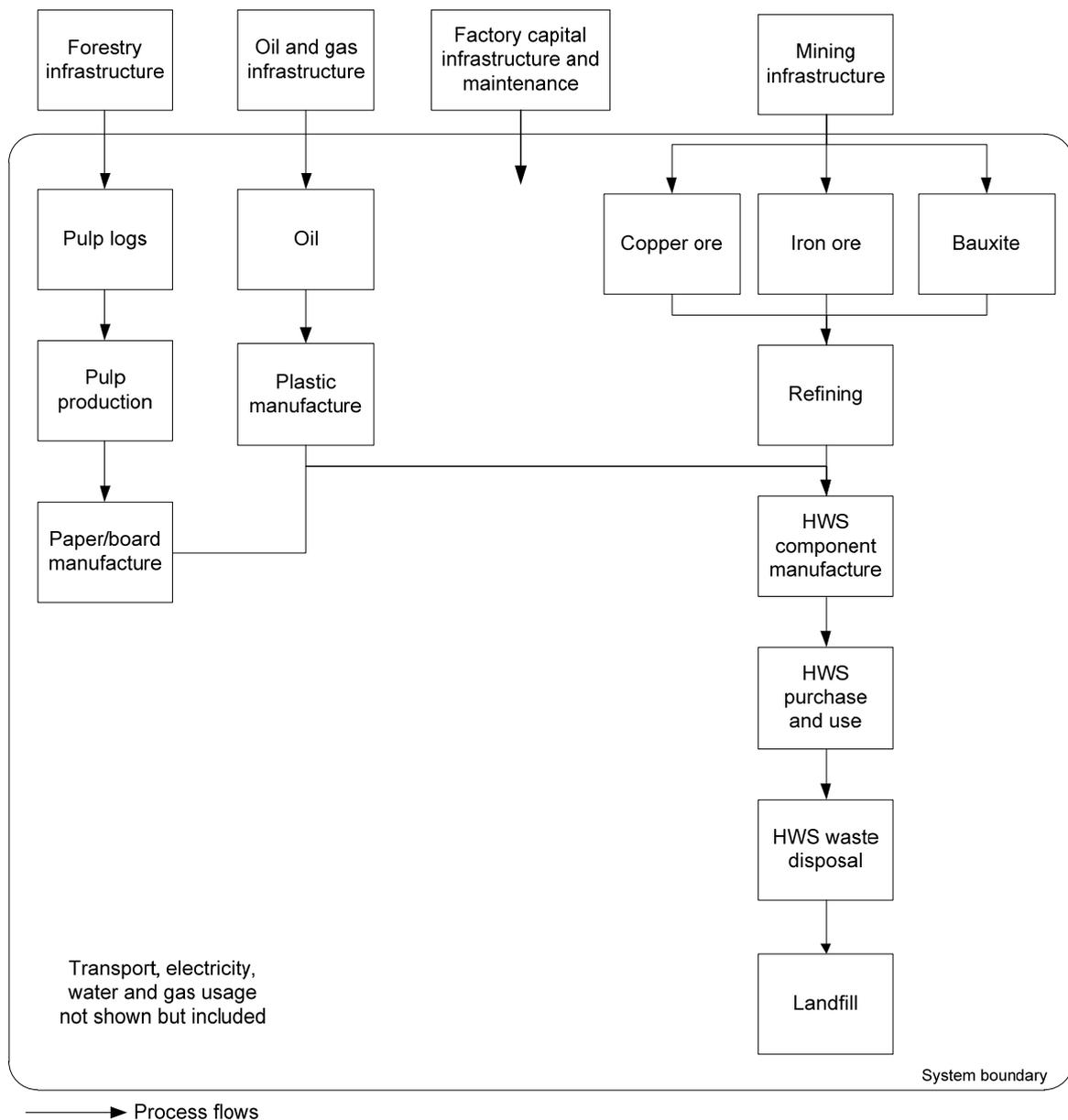
Figure 3-1: System boundary for the hot water systems
