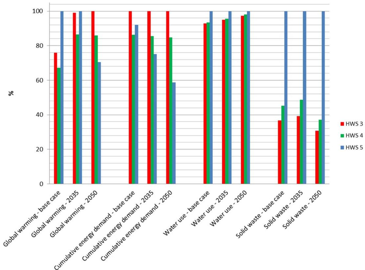
Figure 6-26: Relative summary of electricity grid projections results for Brahe Place (scaled from highest impact) red bar HWS3, green bar HWS4, blue bar HWS 5
