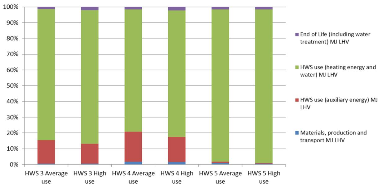
Figure 6-6: Disaggregated % characterisation results for cumulative energy demand for Brahe Place HWSs
