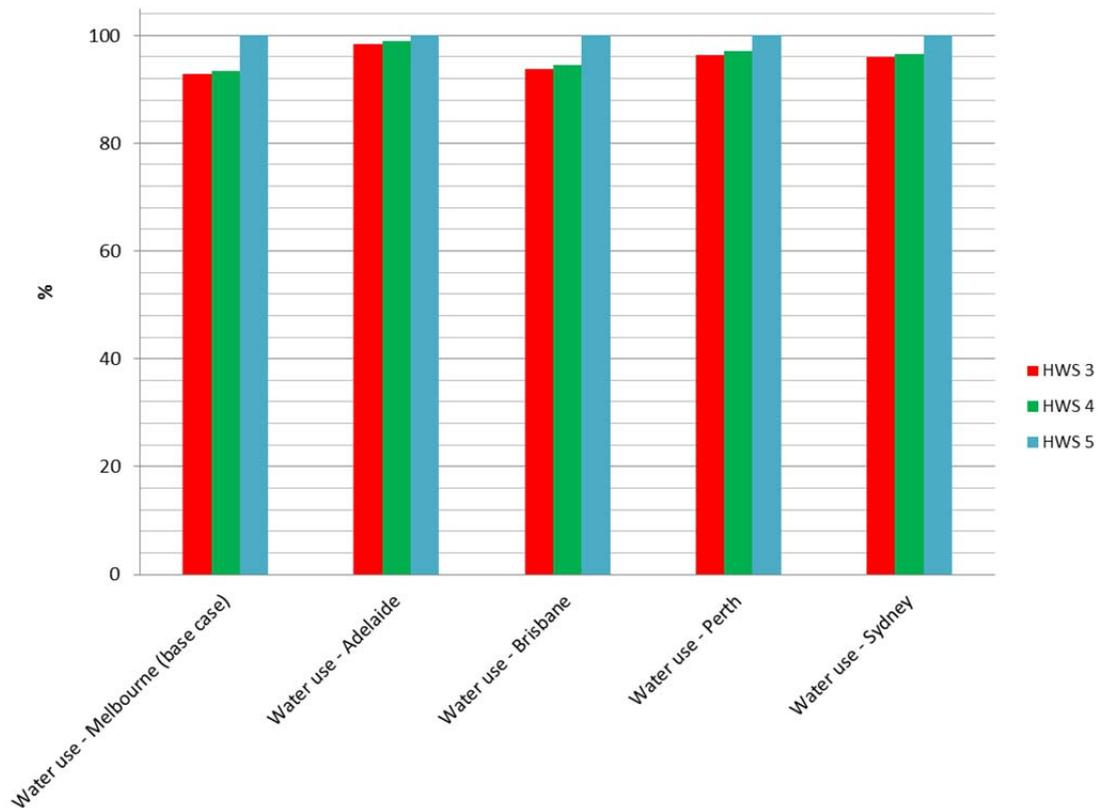
Figure 6-15: Relative summary of sensitivity of regional water use results for Brahe Place (scaled from highest impact) red bar HWS3, green bar HWS4, blue bar HWS 5
