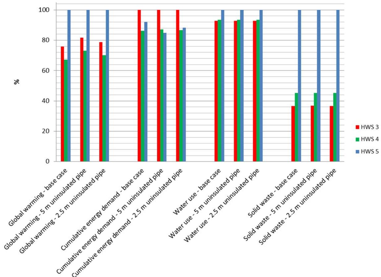
Figure 6-23: Relative summary of sensitivity of extra centralised system loss results for Brahe Place (scaled from highest impact) red bar HWS3, green bar HWS4, blue bar HWS 5
