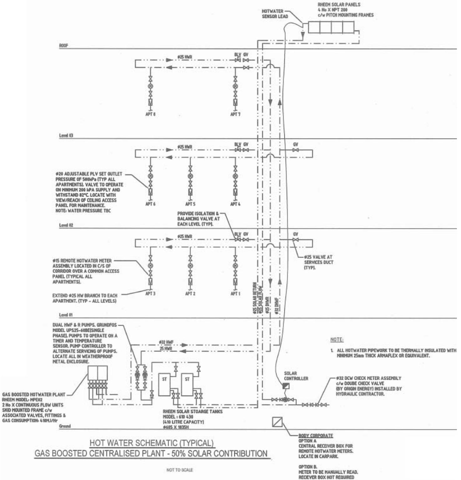
Figure 4-4: Brahe Place building elevation HWS schematic (Wood and Grieve Engineers 2011a)
