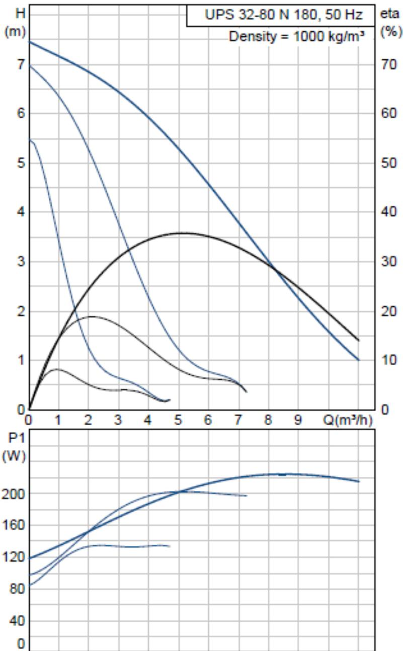
Figure 7-4: Grundfos UPS 32-80 N 180 performance curves (Grundfos 2007a)
