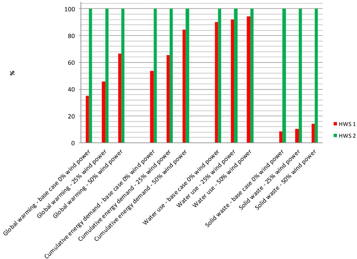
Figure 6-27: Relative summary of green power results for La Banque (scaled from highest impact) red bar HWS1, green bar HWS2
