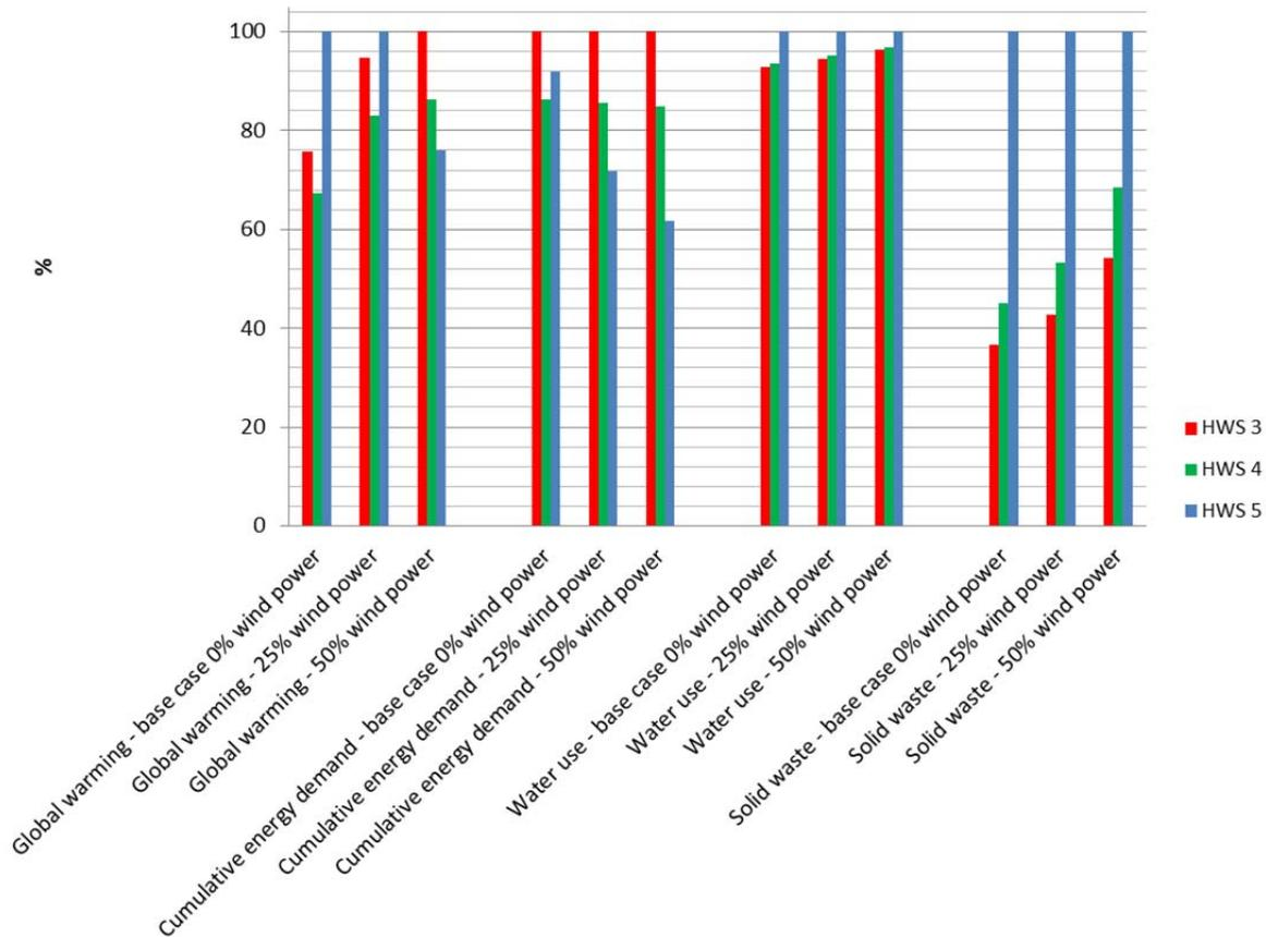
Figure 6-28: Relative summary of sensitivity of green power results for Brahe Place (scaled from highest impact) red bar HWS3, green bar HWS4, blue bar HWS 5
