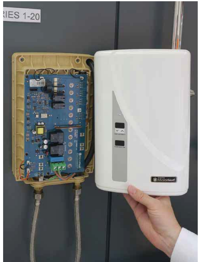
MicroHeat uses electricity to directly energise the water coming into the unit, by using the water as the 'connecting wire' between electrically-energised inert electrodes.
