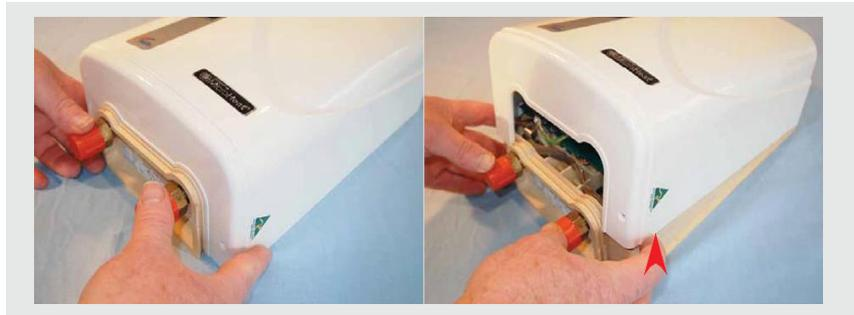
Carefully remove the Display PCB/LED plug and cable connecting either the Display PCB or Indicator LED on the outside of the Exterior Cover to the PCBA.
