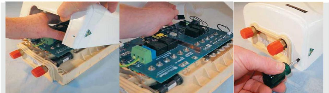
2. Mount the unit onto the wall. Refer back page 23 of manual for mounting screw hole position template and page 19 for product dimensions.
