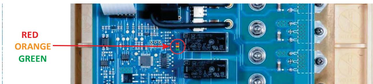
2. Depress the PCBA RESET Button (21) mounted on the PCBA (8).
