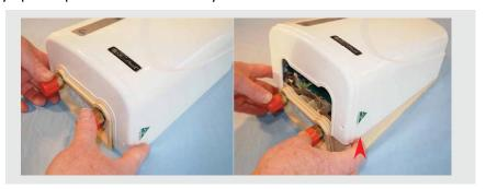
Carefully remove the Display PCB/LED plug and cable connecting either the Display PCB or Indicator LED on the outside of the Exterior Cover to the PCBA.
