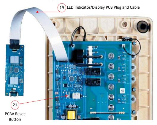
If the error has been successfully RESET, the **GREEN** LED on the PCB will start to flash slowly, indicating the unit is now in standby mode.
